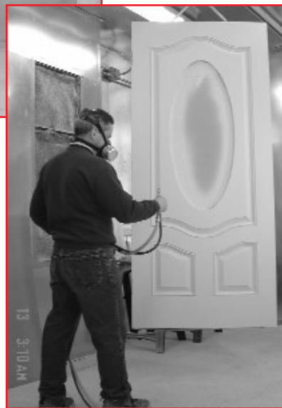
Therma-Tru door getting a finish coat of paint in the stainless steel lined paint booth.
