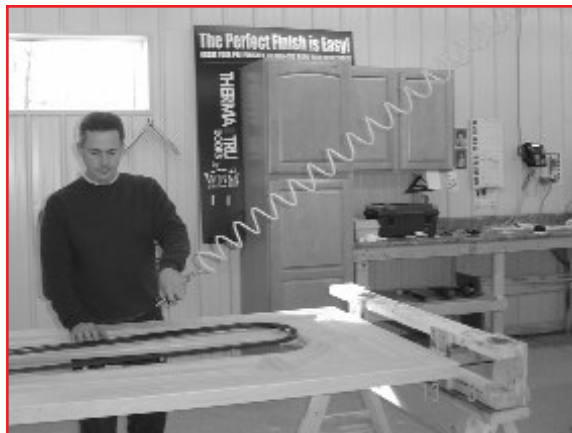
Ray assembles the light frame to complete a pre-finished door.
