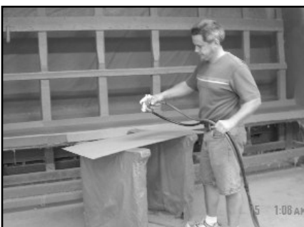
Ray West sprays the laminate sheets with glue before applying to backing.
