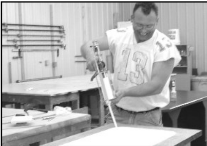
Kevin Grostefon working on an undermount sink application to laminite top.
