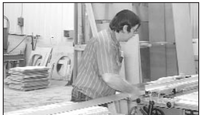
Mike Jones - custom builder for the shop, cutting sheet laminate for a back splash.
