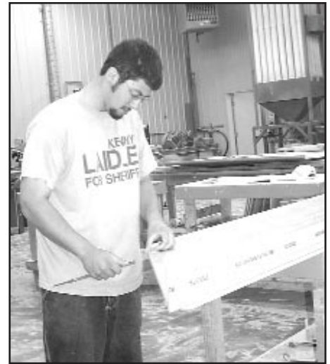
Josh Litherland - filing end cap for finished end.
