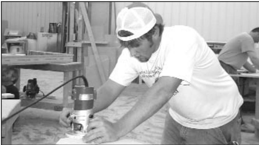
Ryan Kinnett - routing a custom counter top for precision fit.
