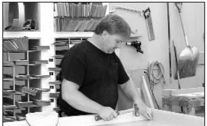
Steve Taylor - setting a miter corner on a right angle counter top.
